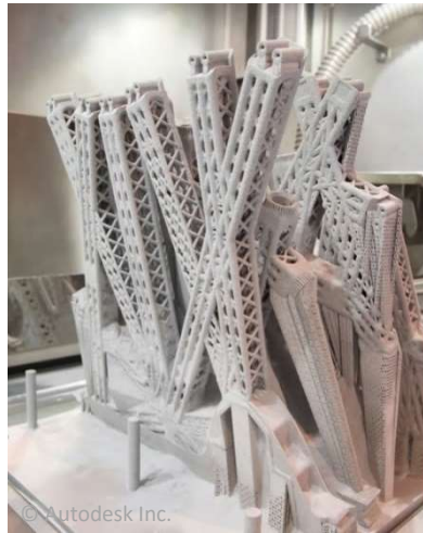
Airbus' AI-designed cabin partition in the 3D printer (left) and assembled (right) [14]. Generative design explored the full design space offered by 3D printing to find this configuration with minimum weight but equal strength.
