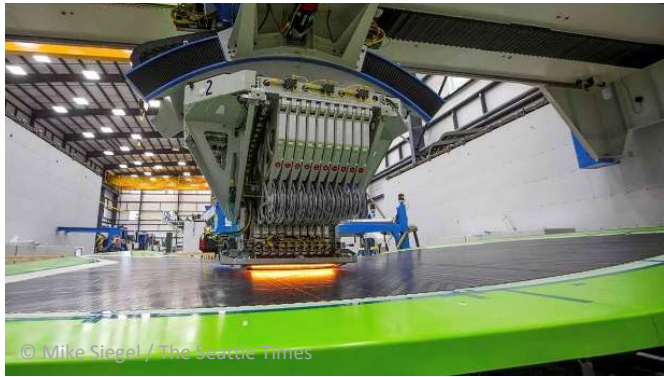
Heated ATL head laying down a wing skin in Boeing's Composite Wing Center [29]. Predicting the part quality and the likelihood of defects that result from a certain pair of part design and machine parameters is a challenge, which is successfully addressed with artificial neural networks.
